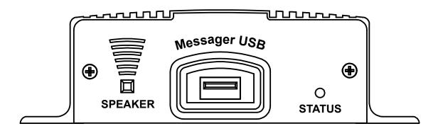
SPEAKER - The SPEAKER switch can be turned ON and OFF to monitor audio playback. The switch has no effect on the audio output connections on the rear of the unit. Switch should normally be kept OFF.
