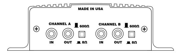
CHANNEL A or B (IN) - This signal level jack allows an external BGM (Background Music) source to be fed through the iLink unit.
