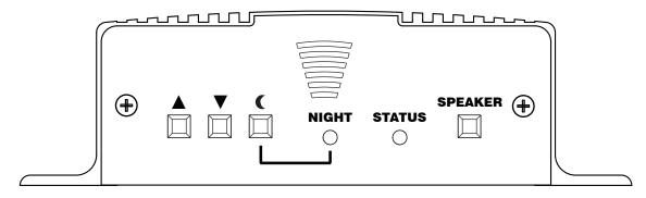
VOLUME UP & DOWN SWITCH - Used to control the  $8\Omega$  and  $600\Omega$  output level of the stored messages.
