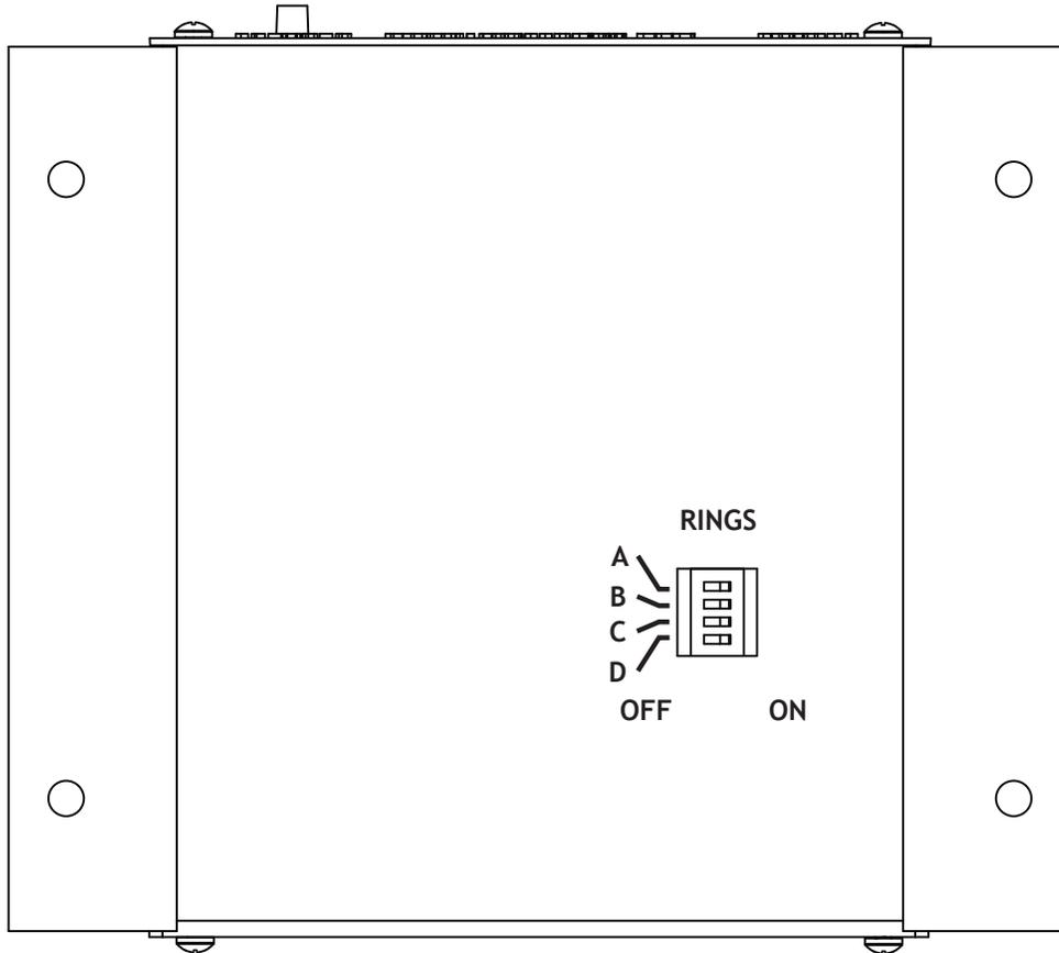
RINGS - These multiple DIP switch positions (A through D) are used to configure the amount of rings required to trigger the night message greeting. Default setting is two rings when all switches are OFF.
