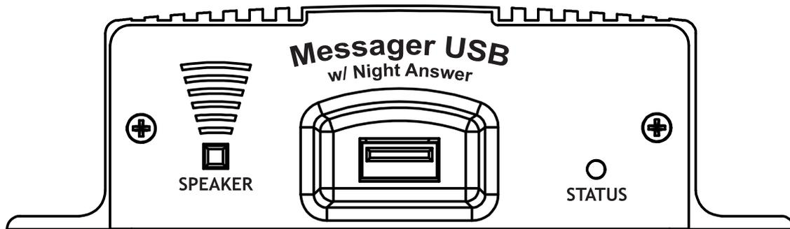
**SPEAKER** - The SPEAKER switch can be turned ON and OFF to monitor MOH and Night Answer audio. The switch has no effect on the audio output connections on the rear of the unit. Switch should normally be kept OFF.
