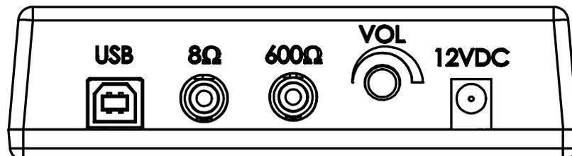
**USB JACK** - This jack is used to connect the Messenger MP3 to a computer via the USB cable supplied.
