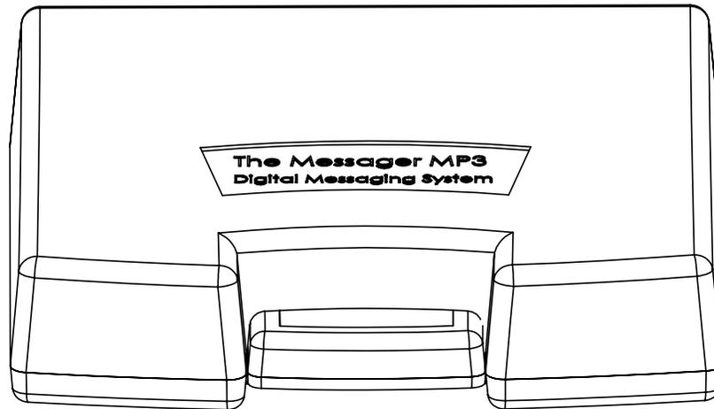
**MESSAGE MATE SLOT** - The slot on the front of the Messenger MP3 accepts a proprietary flash memory cartridge which stores all of the MP3 files.
